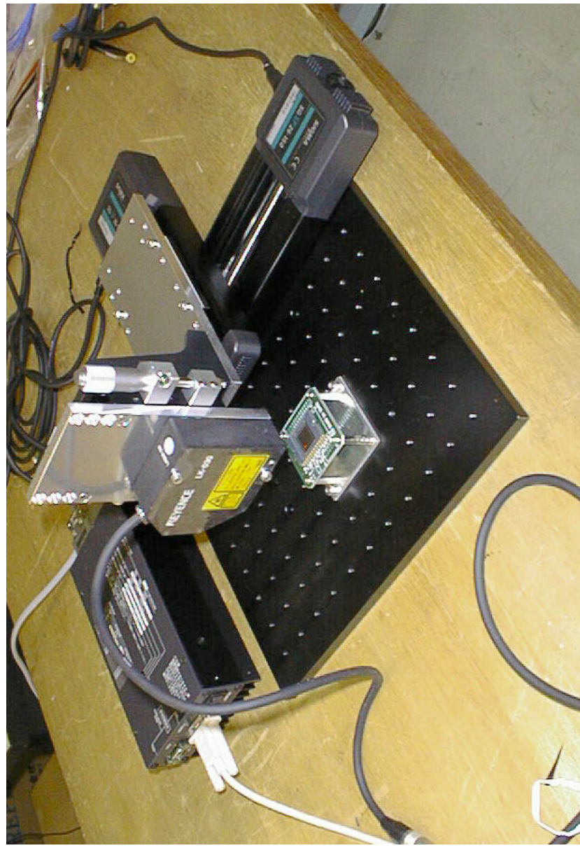
Test setup of X-Y stage and Laser displacement meter
